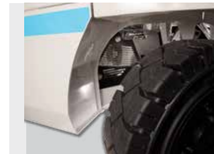
Debris Resistance Package Includes a belly screen and slotted wheel well inserts to prevent larger debris from entering the engine compartment and affecting key components. For additional protection, select the Recycler Package.
