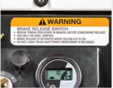
Drive/Tow Switch Electronically releases the parking brake to allow a disabled truck to be moved to a charging station or service area.
