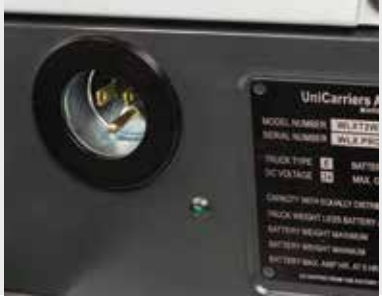
Charger Unit Sealed built-in battery charger option simplifies on-board battery charging.
