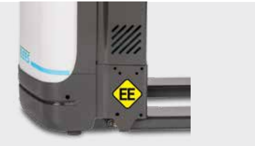
U.L. Type EE Rating Fire safety rated truck for applications requiring Type EE trucks, in accordance with NFPA 505 "Fire Safety Standards for Powered Industrial Trucks"
