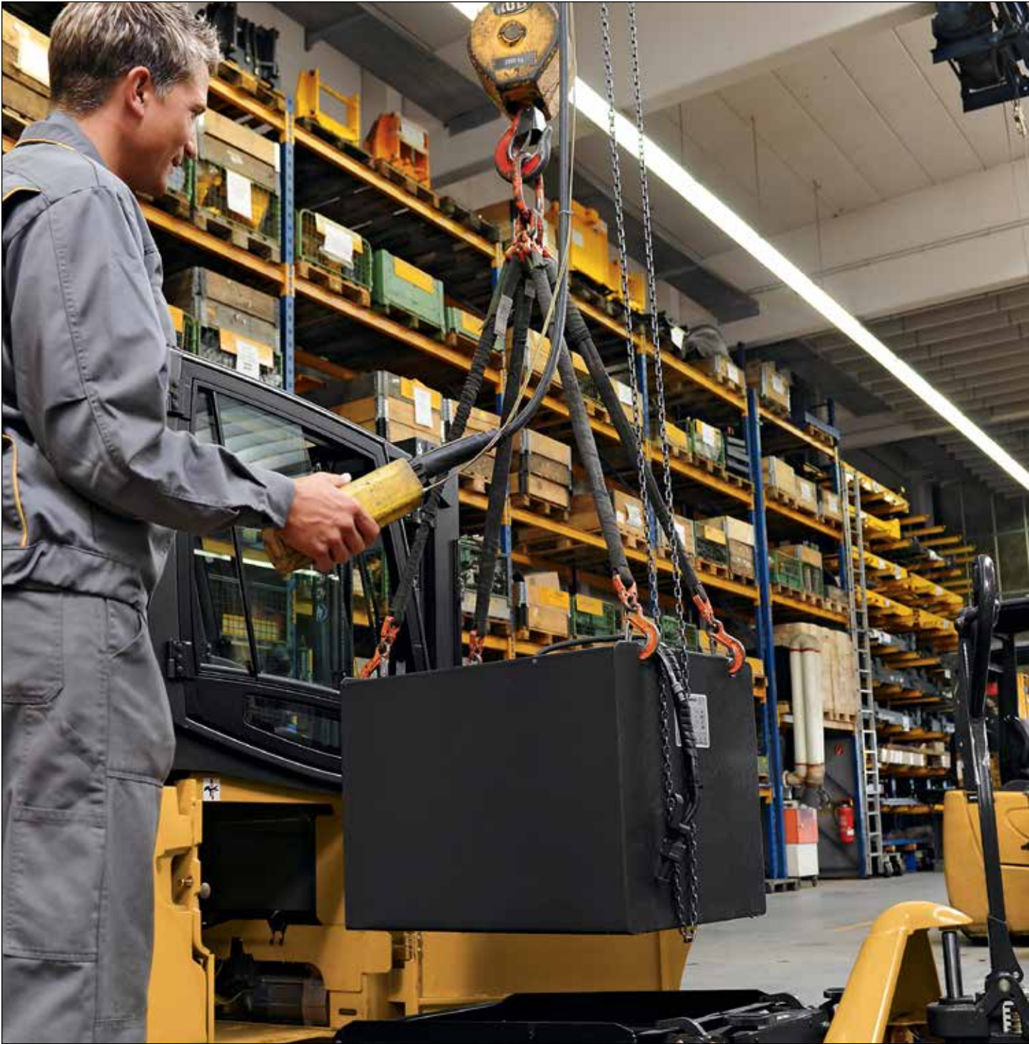
Crane Extraction with SnapFit
